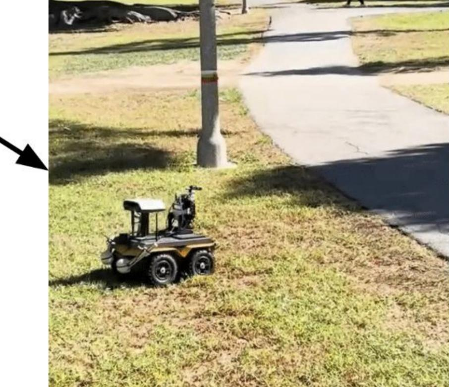
Current cost: Energy expended by wheels Obstacle cost: Time spent around obstacles Slope Cost: Steepness of terrain
